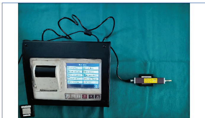
[Table/Fig-5]: Surface roughness evaluation.
